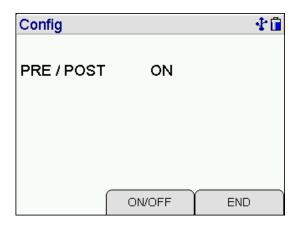
With "ON/OFF" the PRE/POST function can be switched on and off.
