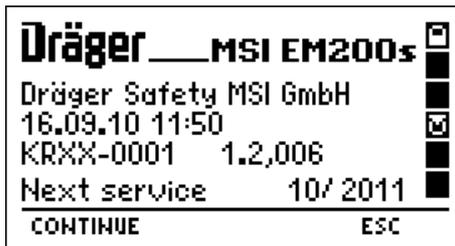
The display informs about the analyser (MSI EM200-s), the manufacturer (Dräger MSI GmbH), the date and time when info function was called, the version of the firmware (e.g. 1.2,006) and the serial number of the analyser.
