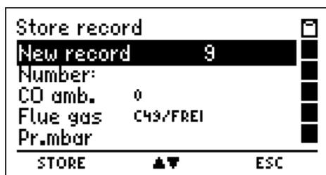
Has no customer ID been selected before measurement, with (STORE) all values may be stored together with date and time. Has a customer ID been selected before measurement (see 11), with (STORE) "New record" all values may be stored under the displayed customer ID.
