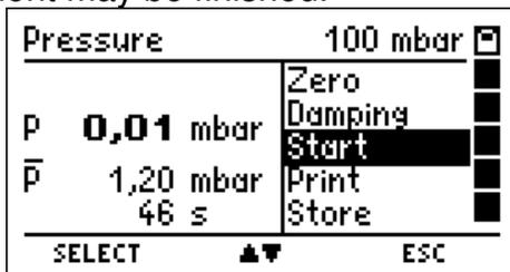
The first value is the actual pressure; the second value is the average of the last measurement. The start-, the stop- and 10 until 20 measurement values between them and the elapsed time have been stored in a buffer. These buffered values may be stored and transferred to a PC. With help of the software "EM Tools" a measurement report including a diagram of the time depending pressure measurement may be printed.
