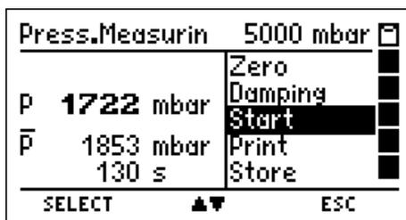
The Start-, the Stop- and 10 until 20 measurement values between them have been stored in a buffer. These buffered values may be stored and transferred to a PC. With help of the MSI PC-program "P7 Tools" you may print a measurement report including a diagram of the time depending pressure measurement.
