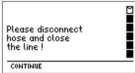
Close the plug of the nipple of the pipe and remove the hose.
