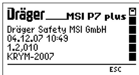
You are informed about the analyser (MSI P7), the manufacturer (Dräger MSI GmbH), date and time (Info Function was called), the version of the firmware (1.2,010) and the serial number of the analyser.
