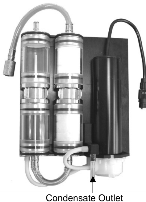
Complete Gas Conditioner with Peristaltic Pump
